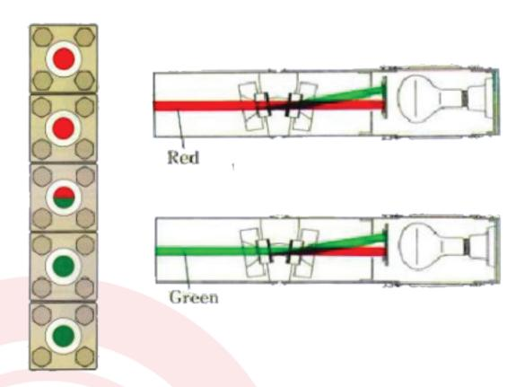
The BN200 series is bi-color boiler water level gauge that meets ASME Section I –Power Boiler requirements, using high quality material and adhering to safety standards. The BN200 Bi-Color water level gauge can handle a maximum pressure of 220 kgf/cm2 (216 barG), and a maximum temperature of 701°F (372 °C).
